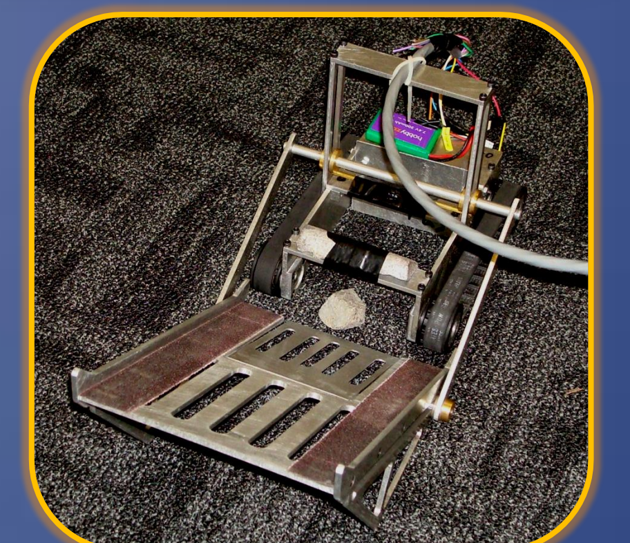
Figure 3. For when the ramp is in front of the rock collection area in the car, there is a one-way gate that allows the rocks to enter it when the ramp goes over it (left). Figure 4. This gate also keeps the rocks from escaping before the vehicle goes over the 4" x 4" again (right).
