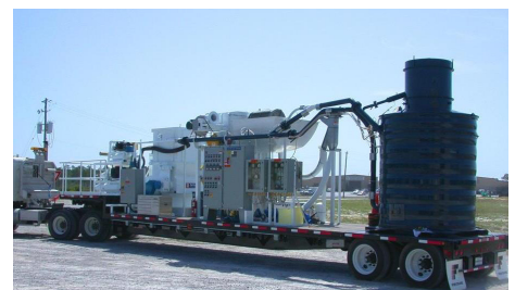
Trailer-mounted furnace for Transportable Waste-to-Energy System
