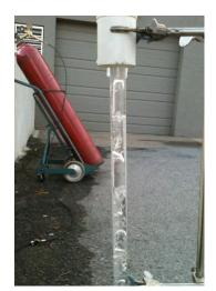
An experiment to verify and qualify Hydrogen-Enhanced Combustion was performed, by allowing pure hydrogen to flow into the air intake of a gasoline-powered generator. A 400-Watt work-light was used as a constant load on the generator, and the fuel consumed, heat generated and air consumed to power the light was recorded. The system overcompensated for the safety concerns regarding hydrogen, and limited the amount of hydrogen delivered such that no change in fuel efficiency was observed.
