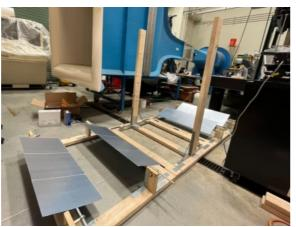
Figure 4: Built solar concentrator.
